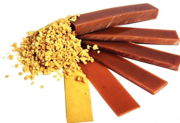
Figure 1. Pellets and cut plates with thicknesses of (from bottom to top) 0.5, 1.0, 3.0, 4.3, 6.1, and 10.6 mm.
