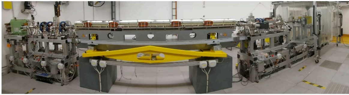
Figure 1: PITZ tunnel annex with installed THz beamline. The electron beam direction is from left to right. Five steering coils are distributed along the undulator to enable gain curve measurements.
