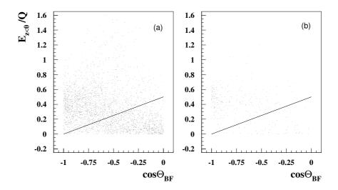
Figure 1: The total energy of the summed calorimeter cluster four momentum vectors in the z < 0 hemisphere of the Breit frame is plotted as a fraction of the event Q against the cosine of the polar angle of the resultant vector, for (a) the low  $Q^2$  and (b) the high  $Q^2$  sample. The line indicates the cut for the secondary analysis described in the text.
