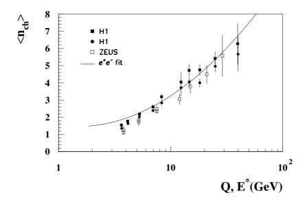
Figure 5: Average charged particle multiplicity in the current region of the Breit frame for data before (solid circles) and after (solid squares) the energy flow selection as a function of Q compared with a parameterisation (line) of one half of average corrected track multiplicities in  $e^+e^-$  events as a function of  $E^*$ . The results of a ZEUS analysis are shown as open squares, with points at the same Q being at different x.
