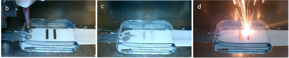
Fig. 1 – Two identical IN625 and S316L multi-material samples (a) were produced by liquid dispersed metal powder bed fusion. The slurries were selectively applied by an automated pipetting system (b), spread across the building platform, resulting in a liquid powder bed and let dry (c) before a laser beam was used to build up the desired geometries layer by layer (d).
