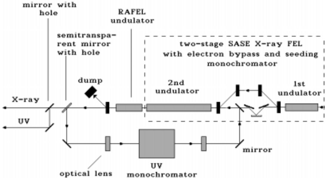
Fig. 1. Schematic layout of the pump-probe facility combining UV regenerative FEL amplifier and soft X-ray FEL at TTF
