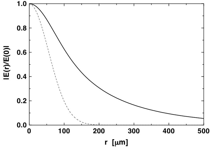
Fig. 5. Transverse distribution of the radiation field amplitude for the FEL amplifier operating at a wavelength of 200 nm. The dashed line is the transverse profile of the electron beam current density,  $\exp[-r^2/(2\sigma_r^2)]$  with  $\sigma_r = 55 \mu\text{m}$
