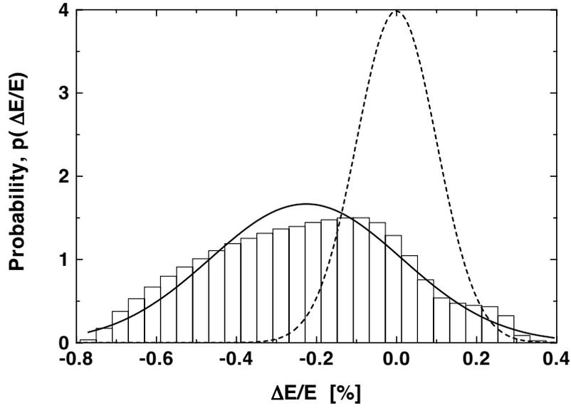
Fig. 3. Histogram of energy distribution of the particles after leaving the VUV/X-ray FEL driven by 1 GeV electron beam. The solid line represents a Gaussian distribution with the rms deviation  $\sigma_E = 2.5$  MeV. The dashed line is the energy distribution at the entrance of the VUV/X-ray undulator ( $\sigma_E = 1$  MeV)
