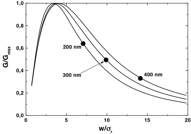
Fig. 4. Power gain in the linear regime versus spot size of the seeding radiation beam (the rms transverse size of the electron beam is  $\sigma_r = 55 \mu\text{m}$ )
