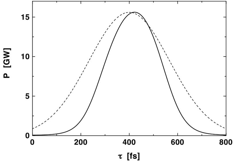
Fig. 7. Temporal structure of the radiation pulse at the exit of the RAFEL undulator. The dotted line represents the longitudinal profile of the electron beam current (the maximum corresponds to 2.5 kA)
