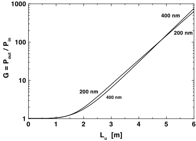
Fig. 6. Power gain,  $G = P_{\text{out}}/P_{\text{in}}$  versus undulator length for the FEL amplifier operating at 200 and 400 nm wavelength (radiation beam size at the undulator entrance  $w$  is equal to 400 and 800  $\mu\text{m}$ , respectively)
