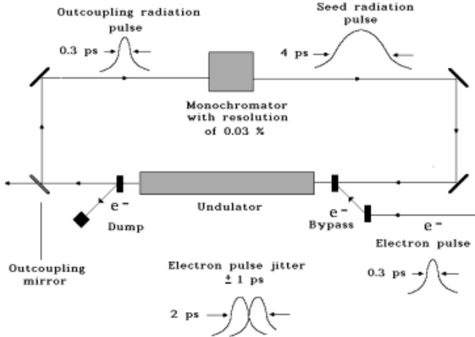
Fig. 2. The use of a monochromator as a pulse stretcher. Drawing illustrates how electron pulse jitter effects on the feedback system can be avoided
