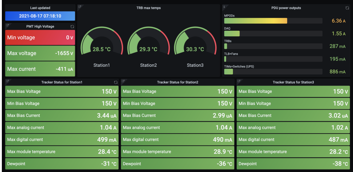
Figure 18. Grafana dashboard of the DCS status overview during an ongoing combined system run. Metrics such as current tracker and PMT voltages, temperatures and power output are shown.
