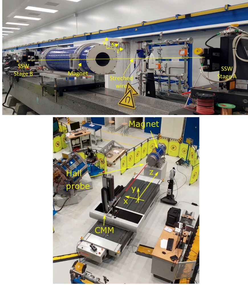
Figure 36. Top: one of the FASER dipoles under measurement using the single-stretched wire at CERN. Bottom: one of the FASER dipoles under measurement using the 3D Hall probe mapper at CERN. (This figure is taken from [62].)
