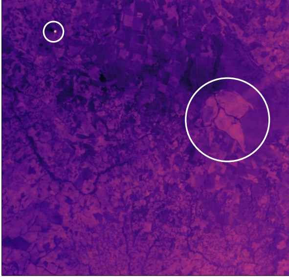
Figure 6: Stitch of two TIR images featuring the first fires detected by the TUBIN spacecraft taken on July, 13th over Brasil at 17:28:30 UTC and 17:28:39 UTC, respectively.
