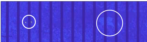
Figure 8: Validation of the location of the first fires detected by TUBIN using a VIIRS image granule taken on July, 13th at 18:00:00 UTC. The image shows VIIRS Band I04 sensitive in the MWIR range of the electromagnetic spectrum.
