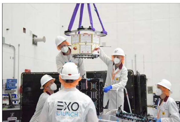
Figure 5: Integration of the TUBIN spacecraft onto the launch adapter five weeks prior to launch in Cape Canaveral. The remove-before-flight items covering solar cells and star tracker optics are still in place (image credit: EXOLAUNCH).
