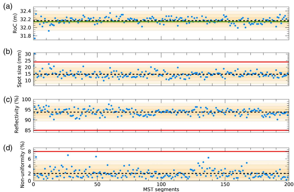
Fig. 6 Main parameters of the produced MST segments, from the first (segment 0) to the last made (segment 199): (a) radius of curvature, (b) D_{80} at twice the NF length, (c) average reflectivity, and (d) reflectivity nonuniformity. In (a), the green solid line represents the reference nominal value; whereas in (c)–(d), the red solid line represents the applicable requirement value. In (a)–(d), the black dashed line represents the average value.
