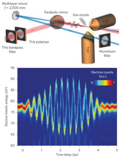
**Figure 5.** Schematic of the experimental setup for a THz streaking experiment at FLASH (top) and the corresponding streaking trace (bottom) recorded as a series of kinetic energy spectra of Kr(4p) photoelectrons produced by a 13.5-nm FEL pulse in the presence of an intense THz field. The energy shift of the electrons as a function of the delay directly represents the vector potential of the THz field. Figure adapted from [45].
