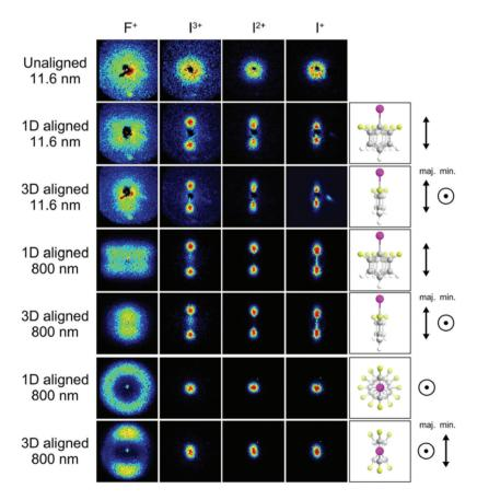
Figure 6. Fragment-ion angular distributions of adiabatically laser-aligned difluoroiodobenzene molecules probed by intense 11.6-nm (107 eV photon energy) FEL pulses as well as by strongfield ionization with an 800-nm laser pulse. The ion images were recorded with a velocity map imaging spectrometer. Figure adapted from [74].
