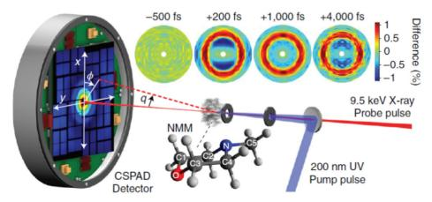
Figure 11. Schematic of a gas-phase ultrafast X-ray scattering experiment on N-methylmorpholine (NMM). The molecules interact with the UV-pump pulse and the hard-X-ray probe pulse in a windowless gas cell inside a vacuum chamber, and the time-resolved scattering images are recorded with a large-area X-ray imaging detector. The insets show difference images of the scattering patterns at several time delays. Figure taken from ([136]).
