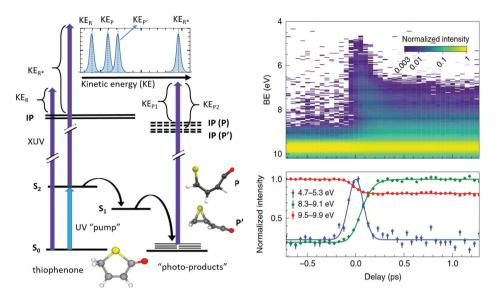
**Figure 10.** Sketch of a UV-pump XUV-probe TRPES experiment on thiophenone (see text). The panel on the right shows the photoelectron spectrum in terms of binding energy (BE), cut right below the outermost-valence level, as a function of pump-probe delay, along with line-outs of the time-dependent photoelectron signal in the BE regions corresponding to ground-state thiophenone (red), photoproducts (green), and thiophenone in the  $S_2$  excited state (blue). Figure adapted from ([125]).
