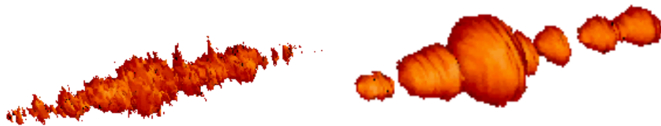
Figure 2.2.4.: Example of the buildup of coherence along the undulator. The left figure shows the radiation intensity profile half way through the undulator, the figure to the right close to saturation. Please note that for a better visualization of the effect the figures were obtained from a simulation that was made at longer wavelengths and for a coherence length L_c which is 10% of the electron bunch length L_b , whereas for XFELs the typical ratio is L_c/L_b \simeq 10^{-3} .
