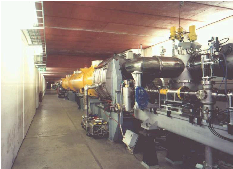
Figure 2.2.2: View into the TTF Linac tunnel. The electron beam (already accelerated by the capture cavity) comes from the right and is injected into the first accelerator module, which can be seen in the background (yellow vessel).
