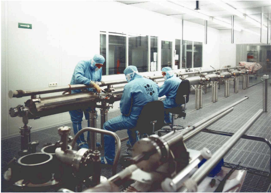
Figure 1.1.3: Assembly of a string of eight 9-cell cavities in the clean room at TTF.
