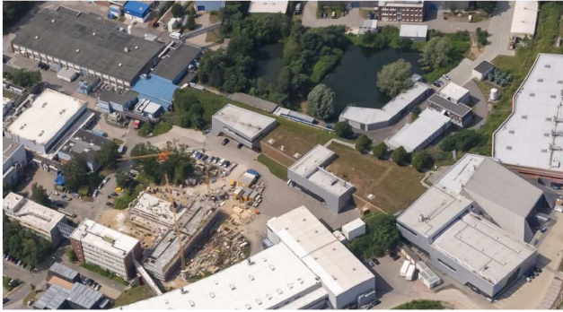
Fig. 1 Aerial view of the FLASH facility in the DESY campus. Electrons are generated in the hall on the top left and are fed into the grass-covered tunnel. At the bottom right, the Albert-Einstein experimental hall of FLASH1 and below the Kai-Siegbahn experimental hall of FLASH2 are visible. FLASH crosses the PETRA ring in between two experimental halls at the bottom center and on the top right.
