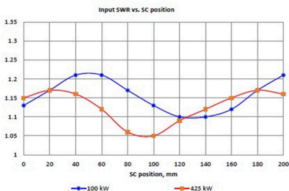
Figure 3: SWR vs. short circuit position of an isolator at different power levels.
