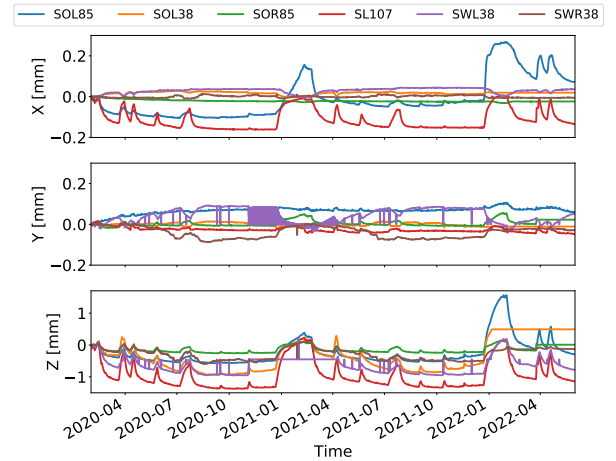
Figure 5: Measured movement between tunnel segments at the six measurement stations between SOL85 and SWR38, locations are indicated in Fig. 1. These measurement devices were installed later compared to the ones in Fig. 4, and are only operated since February 2020.
