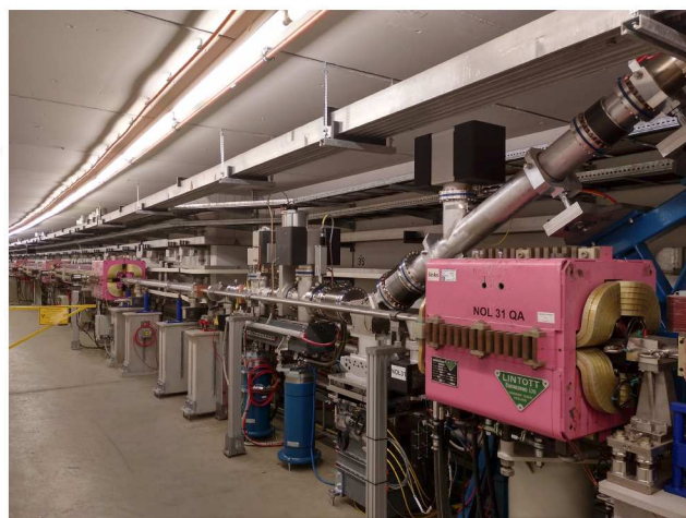
Figure 2: Dipole magnet and front-end components of the dipole beam P66 in the PETRA III tunnel.
