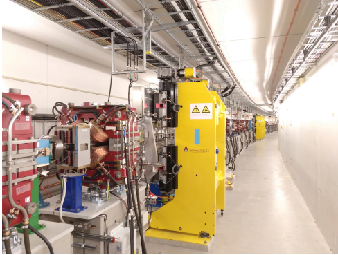
Figure 4: Undulator and front-end components of beamline P62 in the PETRA III tunnel of the Paul P. Ewald hall (installed in 2020).
