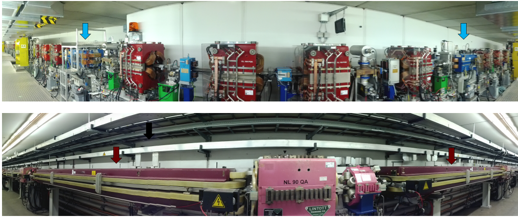
Figure 2: Panoramic view of a DBA cell in the Max von Laue hall (top) and a FODO cell in an arc of the PETRA III ring (bottom). The arrows indicate the location of the dipole magnets.
