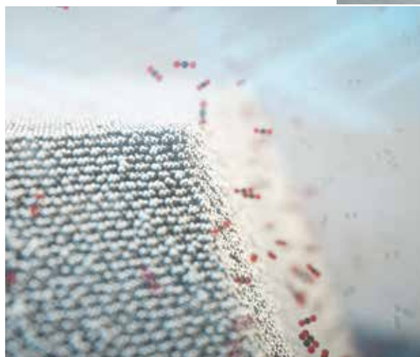
On the surface of the nanoparticle, carbon monoxide oxidises to carbon dioxide.
