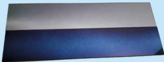
An uncoated (top) and nanopaper-coated silicon wafer. The nanocellulose layer is only 200 nanometres thin. The wafers are each two centimetres wide and ten centimetres long.
