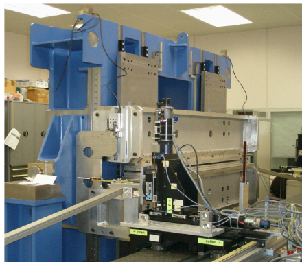
Figure 2: U48 at hall probe measurement bench.
