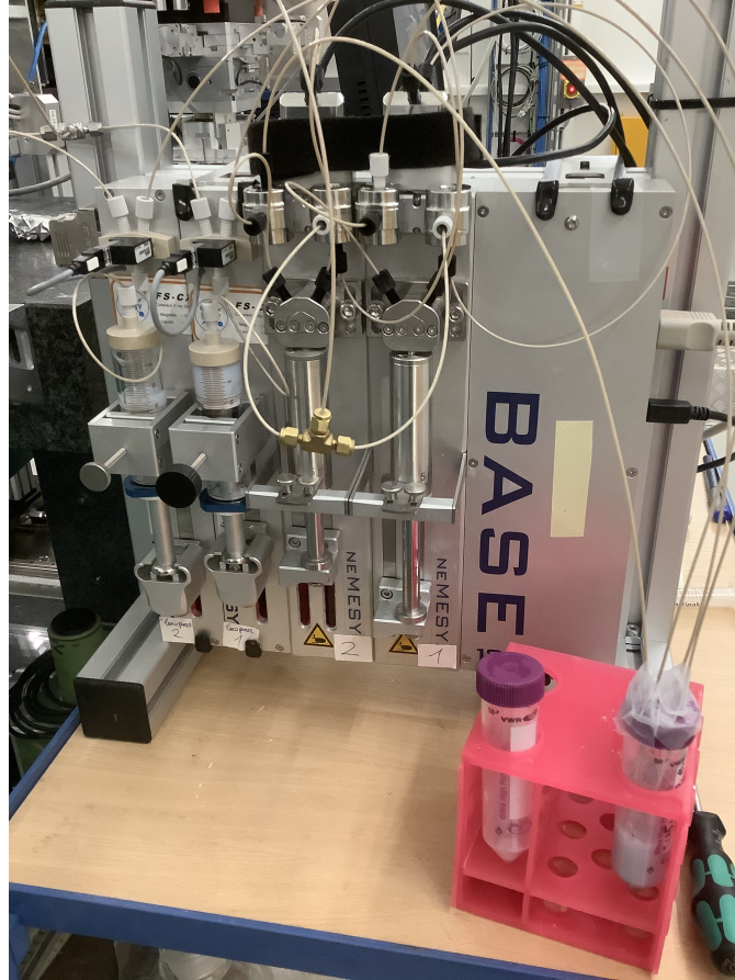
Figure 4.8: Installation of the pumping system driving the jetting at the beamline P10 at PETRA III.
