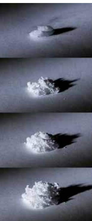
When HDA ice is converted into LDA ice, the volume of ice spontaneously increases by about a quarter.
