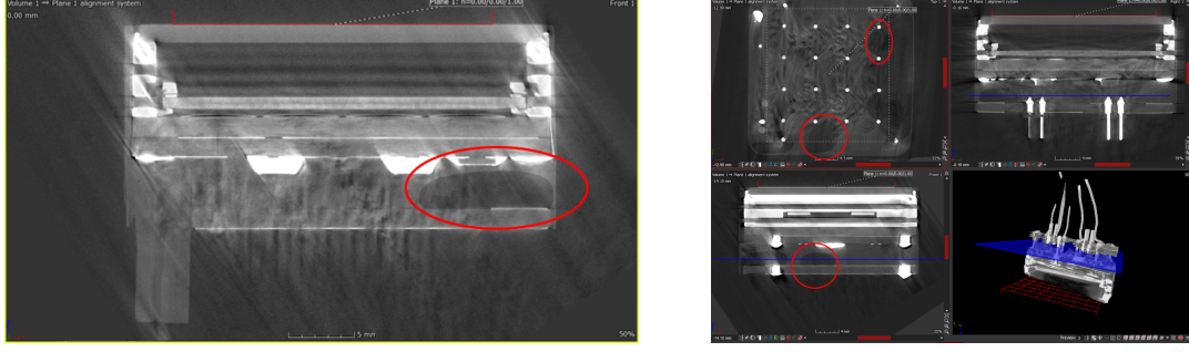
Figure 9. 3D X-ray scan of one of the Photonis XPM85212 MCP-PMTs in order to identify eventual weak points leading to repeated failures of MCP-PMTs when operated in vacuum. Some of the air bubbles are depicted by red ovals. Copyright 2020 CERN for the benefit of the ATLAS Collaboration. CC-BY-4.0 license.
