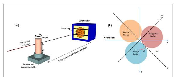
**Figure 1.** SAXS-CT experiment. (a) Schematic representation of the experimental setup for SAXS-CT; (b) top view of the sample assembly as the specimens were mounted and the coordinate system of the experiment. A detailed description of the instrument is presented by Roth and coworkers (Roth *et al* 2006).
