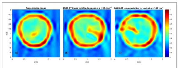
Figure 5. Comparison between transmission and small-angle scattering images. (a) reconstructed transmission image; (b) SAXS-CT reconstructed image for the specific momentum transfer  $(q_1 = 0.94 \text{ nm}^{-1})$  and, (c) for the momentum transfer  $(q_2 = 1.46 \text{ nm}^{-1})$ . The color bar label '1' refers to the highest scattered photons intensity, while '0' indicates no detectable scattered photons at the respective position in linear scale.
