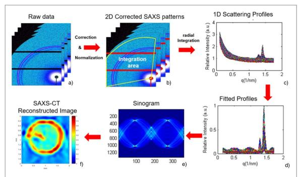
**Figure 2.** SAXS-CT reconstruction. Successive steps of SAXS-CT data treatment and image reconstruction. The acquired 2D SAXS patterns (a) are corrected, normalized and then radially integrated (b). The following 1D profile (c) is fitted by iterative least-square routine and the resulted profile (d) is used to generate the sinograms for each value of q-vector (e). Using the standard FBP algorithm, the SAXS-CT tomogram is reconstructed for each q-vector (f).
