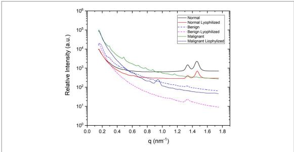
**Figure 4.** Comparison between the SAXS scattering profiles of normal, benign and malignant breast specimens at normal and lyophilized states.
