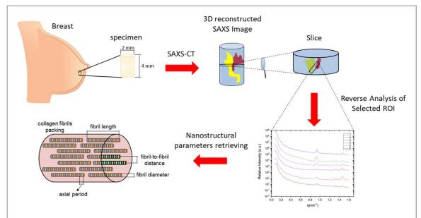
**Figure 3.** SAXS-CT length scale. Schematic representation of the approach for the nanostructure resolving microscopy of macroscopic soft tissue specimens. Here is presented the application on monitoring the hierarchical arrangement of fibrillar collagen in a macroscopic breast specimen. Information such as collagen fibrils packing, fibrils length, fibril diameter, fibril-to-fibril distance and axial period can be accessed.
