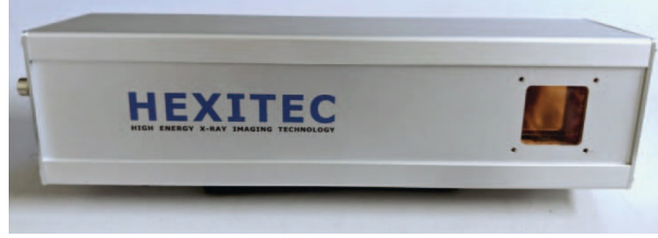
Figure 5.12: Image of the HEXITEC detector (from [175]). The active area of the chip is visible on the right side of the detector. For the experiments, the detector chip was covered by a 1.5\text{ mm} thick aluminium plate to reduce the flux of low-energy X-rays on the detector chip.
