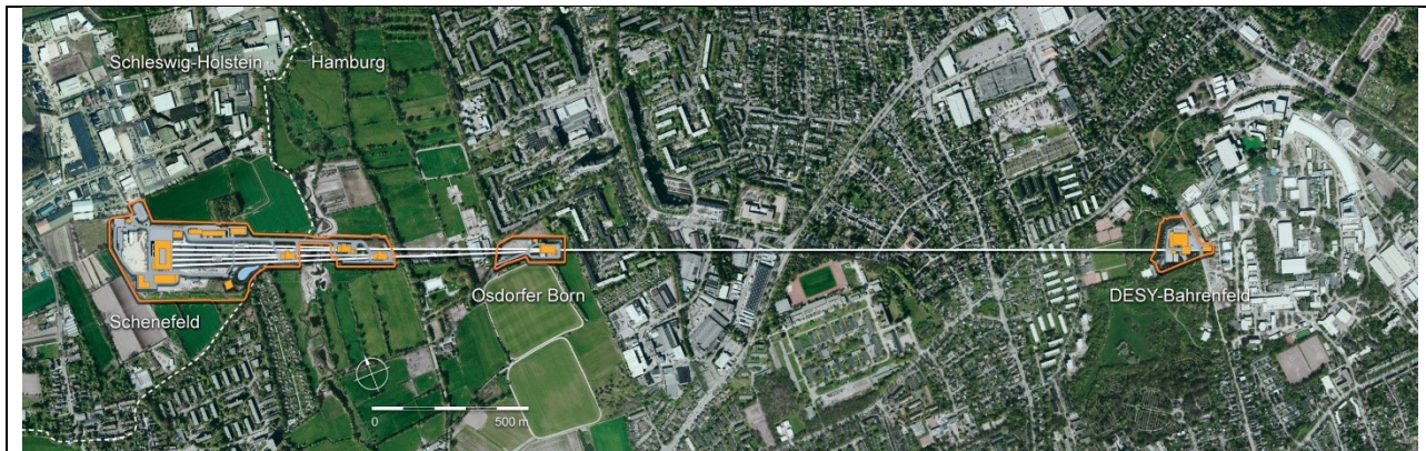
Fig. 1: Bird's-eye view of the facility showing the location of the tunnel buildings in the urban area of the city of Hamburg. The injector is on the right on the DESY campus, while the experiment hall and headquarters of the European XFEL are on the left in the federal state of Schleswig-Holstein. Note the fan of five photon beamlines entering the experiment hall.
