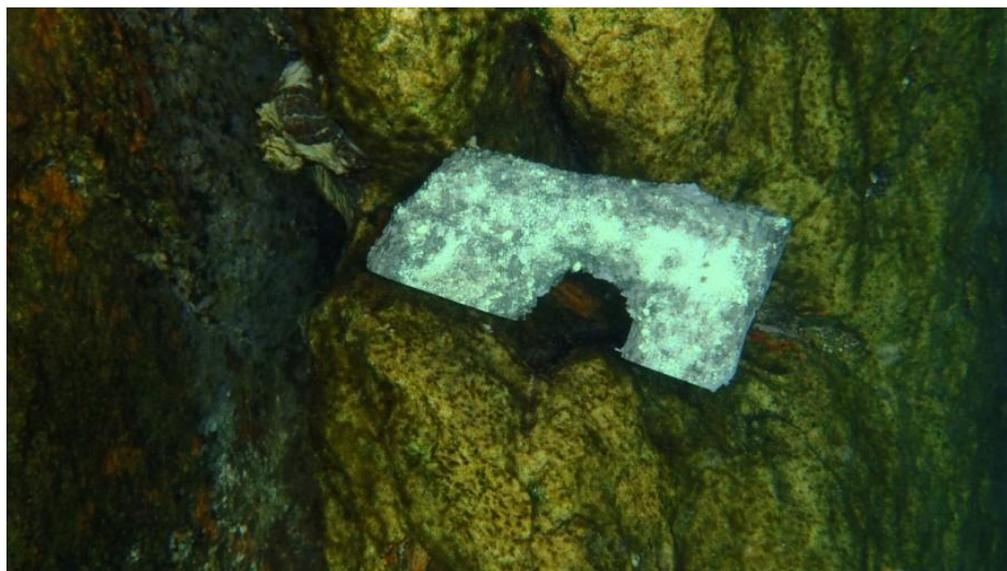
**Fig. 27.** Blue–green color luminescence of  $\text{SrAl}_2\text{O}_4:\text{Eu}^{2+},\text{Dy}^{3+}$  at a depth of 5 m under real sea conditions.
