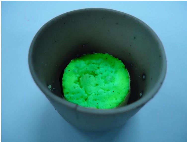
**Fig. 2.** Bright luminescence of  $\text{SrAl}_2\text{O}_4:\text{Eu}^{2+},\text{Dy}^{3+}$  based phosphor in the open air under sun light excitation.
