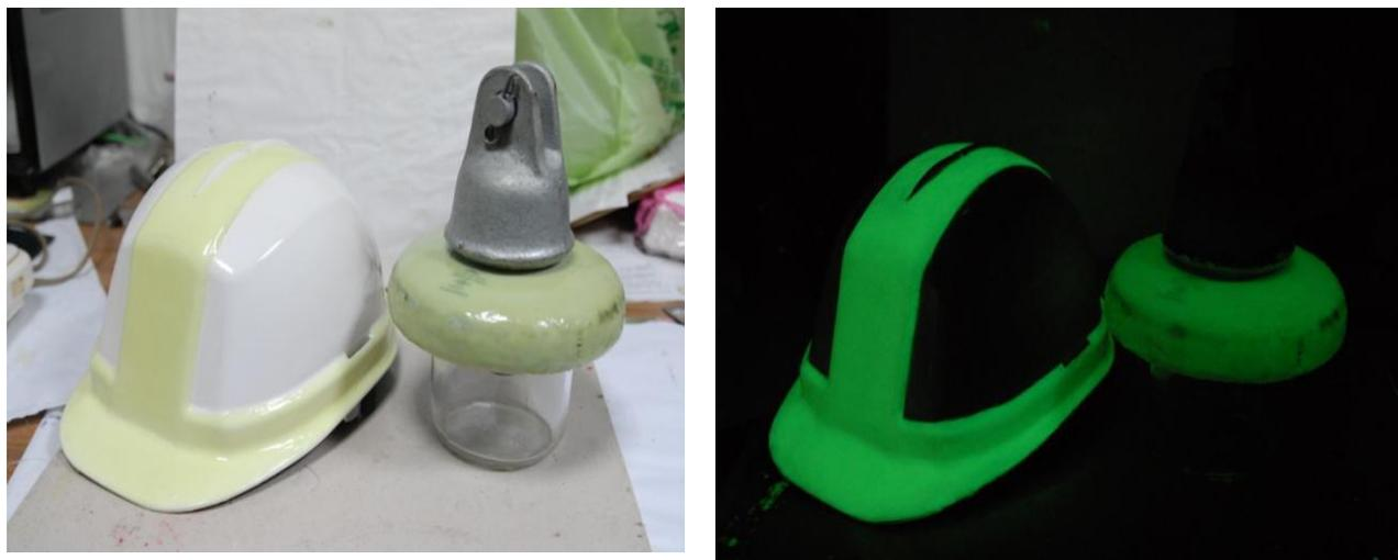
**Fig. 25.** A helmet and a high-voltage insulator (ceramic) in the day time and at dark.
