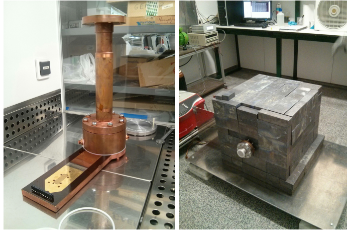
Figure 32. Left: Photograph of the detector chamber assembled on the readout support, both made of copper. The detector is coupled to a copper interface tube for coupling to the optics system. The high density rectangular connector for the connection to the front electronics can also be seen in the middle of the gold plated zone in the readout support. Right: Photograph of the detector surrounded by the lead shielding.
