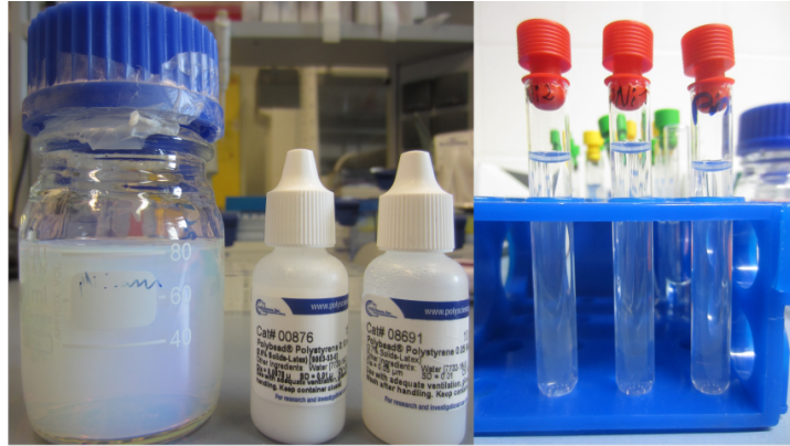
Figure 3.6: Polystyrene and pNipam sample systems. Left: pNipam and polystyrene spheres with R = 50\text{nm} and R = 25\text{nm} . Right: Strongly diluted pNipam samples in glass capillaries.
