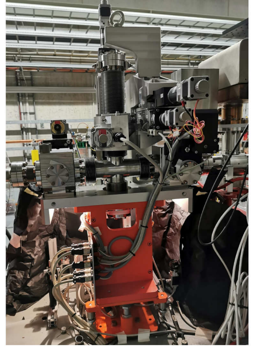
Figure 3: Installed collimator device. An adjustable support allows precision alignment to the beamline. Cameras observe the collimator position through window flanges from underneath. All collimators can be adjusted remotely.
