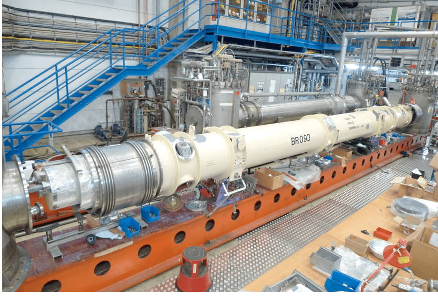
Figure 8: Remaining bench for cryogenic tests of HERA dipoles with a dipole on the bench. Note the open sliding sleeve connection of the vacuum vessel to the cryogenics end box.
