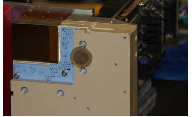
Fig. 7. The sensor mounted on the supporting LTCC and undergoing testing
