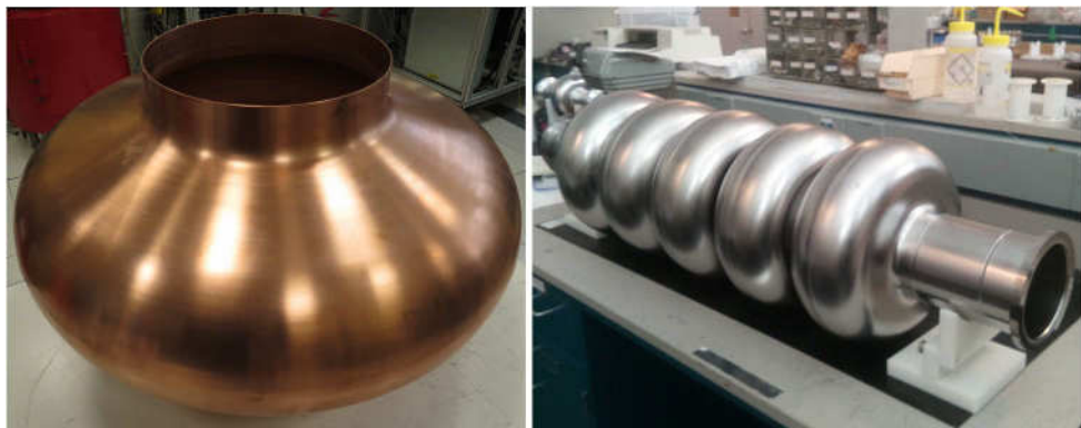
Fig. 3.16. Left: A FCC seamless single-cell 400 MHz Cu prototype cavity for Nb on Cu thin-film coating, fabricated at INFN Legnaro National Laboratory (Italy). Similar cavities will be used for operation at the Z pole. Right: A prototype FCC five-cell 802 MHz bulk-Nb cavity for t\bar{t} operation, fabricated and tested at Jefferson Lab (USA) [304].
