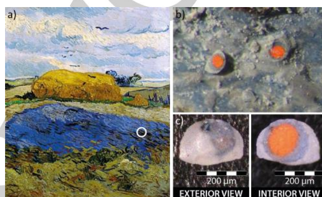
Figure 1. a) Photograph of Wheat stack under a cloudy sky by Van Gogh (October 1889, oil on canvas, Kröller-Müller Museum, NL). The sample area is indicated by the white circle; b) Detail of the severed pustular mass on the painting surface; c) Detail of the paint sample.
