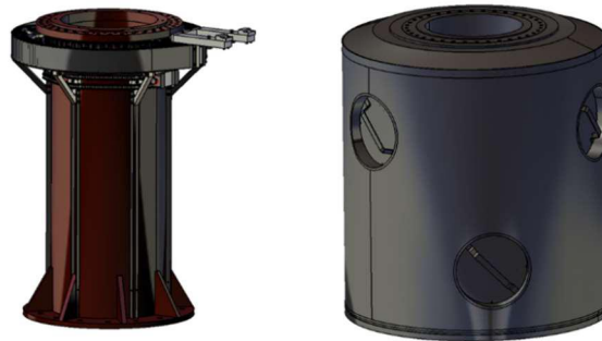
Figure 14. CAD views. On the left, pGCT tower with cable wrap. On the right, GCT pre-production tower design.
