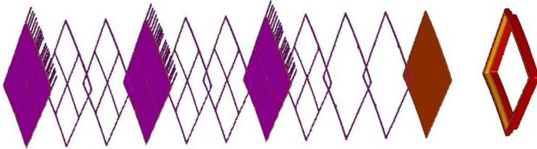
Figure 7.1: Exploded view of the GridGEM module showing the different components stacked one after the other. From the right it is possible to see the back-frame, followed by the PCB, 3 ceramic components spacing the first GEM of the stack. The other 2 GEM are similarly spaced by other ceramic components including a grid shaped inner element to reduce the sagging of the foils due to the electromagnetic and gravitational forces involved.
