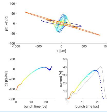
Phase space simulation for SLMbased bunch shaping
