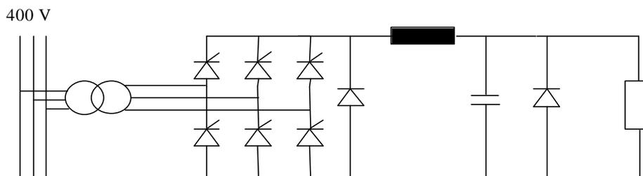
Fig. 4 Schematic of a 3 phase SRC bridge with passive filter
