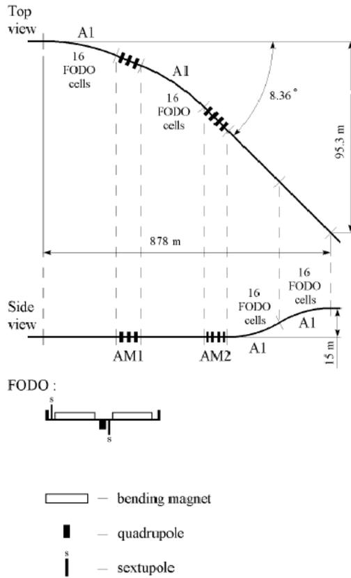
Fig. 7: Magnet lattice of the beam elevation system
