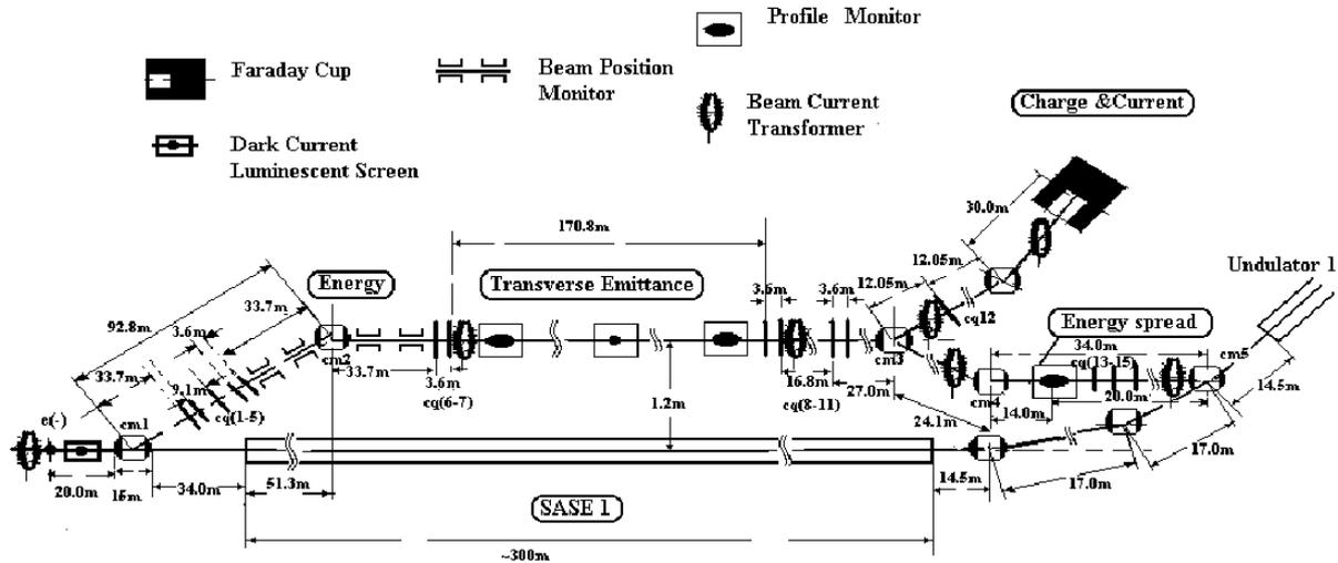
Fig. 9. Lattice of the diagnostic commissioning line
