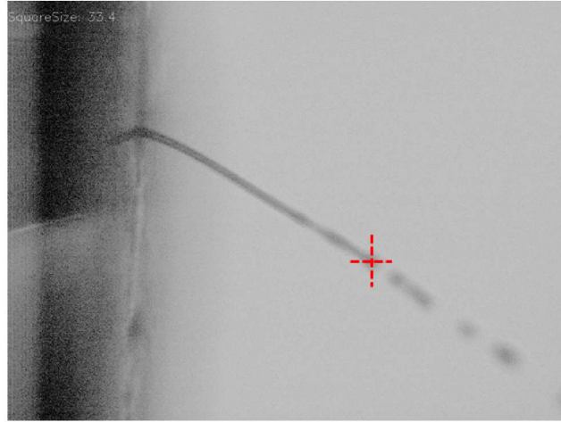
Figure 7.16: High magnification microscope image taken during the experiment. The red cross represents the beam position at \text{Jet}_y = 350 \mu\text{m} .
