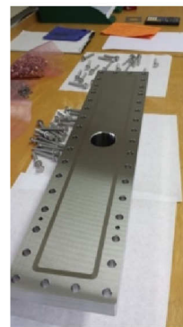
Figure 4: A special vacuum test adapter for all principle tests and for the final acceptance test like rest gas analysis and leak check.
