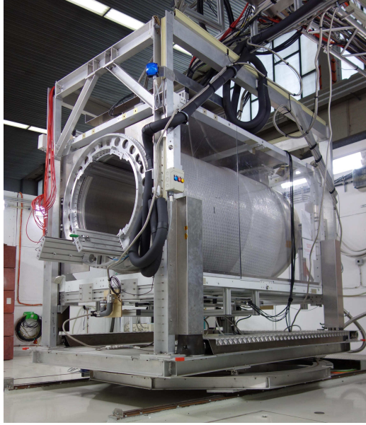
Figure 20: TB24/1 test beam area at DESY: movable lifting stage with the PCMAG 1 T solenoid.
