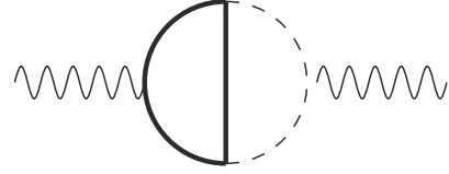
FIG. 3. The master integral K_{14} . Massive (massless) propagators are represented by solid (dashed) lines. The presence of a massless cut determines the asymptotic behaviour K_{14} \sim \log(1-x) .
