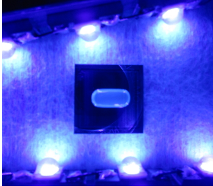
Figure 8.2: ATLAS07 miniature sensor with DYMAX 3013 glue exposed to UV light: the glue becomes fluorescent under UV light exposure.
