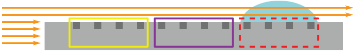
Figure 8.4: Scheme of a fluorescence measurement of a strip sensor with glue (not so scale): a beam is pointed at the sensor perpendicular to sensor strips (dark grey). While strips at the sensor edge (yellow area) are expected to see hits while the beam is pointed at the sensor, photon absorption inside the silicon will prevent strips further away from the sensor edge from registering hits (violet area). Strips beneath glue (red area) are thus expected to see hits only when the beam is pointed at the glue and if fluorescence occurs.
