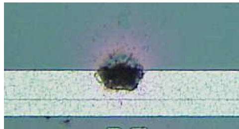
Figure 6.35: Residue of silver paint (diameter about 80\text{ }\mu\text{m} ) on the surface of an ATLAS mini sensor. The burnt area surrounding the silver paint indicates a previous high current.
