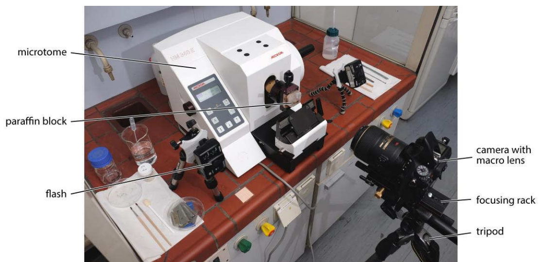
Fig. 2 Setup for episcopic microtomy, lens hood removed
