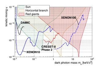
Figure 1: Parameter space for the kinetic mixing between dark photons and standard model photons. Shown in *red* are the exclusion limit for CRESST-II phase 2 obtained with the detector module Lise in comparison with results from LXe and Si based experiments together with constraints from anomalous energy loss in stars. For references see [10].
