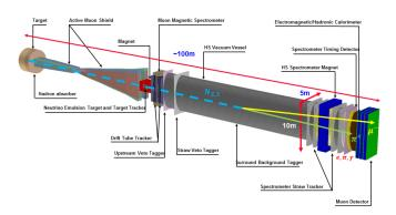
Figure 3: The SHiP detector
