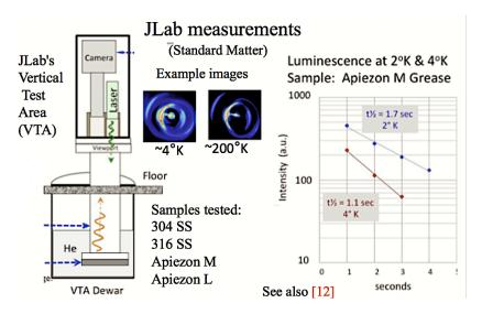
Figure 3: Temperature dependent luminescence.
