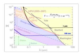
Figure 1: Projected aKWISP coverage in the parameter space of a Yukawa-type interaction between two macroscopic bodies.  $\alpha$  and  $\lambda$  represent the interaction strength and range, respectively. The black curve refers to a 1  $\mu$ m separation distance between the two DMIM membranes, while the blue curve refers to a 100 nm one (see also text). The background plot is taken from [4].
