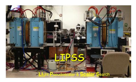
Figure 5: Image of the LIPSS experimental setup at Jefferson Lab. The dipoles are colored light blue and can be joined to form a 2 meter long, 1.7 Tesla B-Field.
