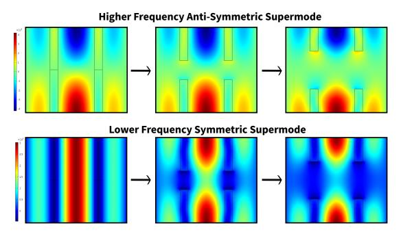
Figure 3:  $E_z$  field for a  $TM_{031}$ -like mode (top) and a  $TM_{030}$ -like mode (bottom). A dielectric ring is placed to suppress the out of phase field, and as the ring is split the frequency of the  $TM_{030}$ -like mode tunes upwards towards the  $TM_{031}$ -like mode.
