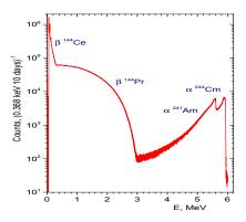
Figure 3: The spectrum of <sup>144</sup>Ce-<sup>144</sup>Pr measured with the Si(Li) detector.
