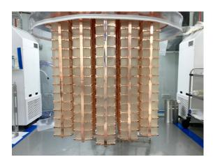
Figure 3: The CUORE array of 988  ${\rm TeO_2}$  Bolometers in 19 towers prior to installation in the cryostat. All crystal axes are nomonaly equally oriented with small uncertainties.
