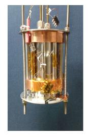
Figure 2: Nb cavity instrumented before the insertion in the LHe criostat.
