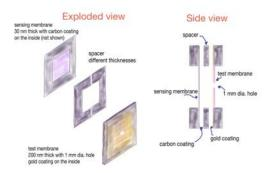
Figure 2: Sketch of the Double Membrane Interaction Monitor (DMIM) (see text).
