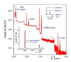
Figure 2: The spectrum of  $^{207}$ Bi source measured with the Si(Li) detector in energy range of (0.01-2.0) MeV. The inset shows the electron peaks corresponding to internal conversion from K-, L-, M-shells of the 570 keV nuclear level.
