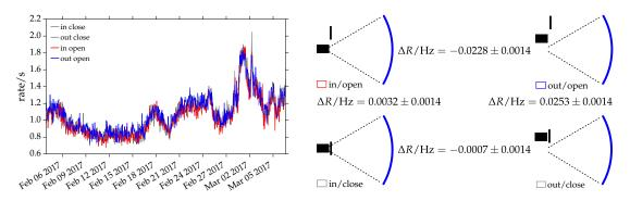
Figure 4: Left: observed pulse rate in one of the measurement runs. Right: A measurement is composed of many event cycles, where in each cycle four different 60-second measurements are performed. The schematic show these four different combinations obtained with open/closed shutter and with camera in/out.
