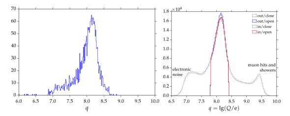
Figure 3: Left: Charge distribution for a flasher run with very low power setting and, therefore, composed mostly by single photo-electrons. Right: Charge distribution observed in one of the measurement runs. Note that in both cases  $q = \lg(Q/e)$  where Q is the charge of a pulse.
