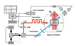
Figure 1: Schematics of CAPP magnetometer.
