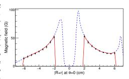
Figure 2: Magnetic field as a function of radial position |R+r| at  $\theta=0$ . Dashed (blue) lines are obtained from the finite element method and correspond to the toroidal cavity system, and solid lines (red) correspond to the cavity tube. Dots with error bars are measurement values. The results at positive R+r are along a coil, while those at negative R+r are between two neighboring coils.
