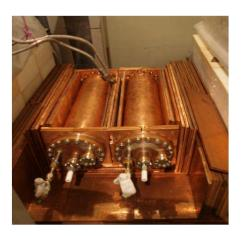
Figure 1: A large proportional counter (LPC) with a casing of copper inside passive shilding.
