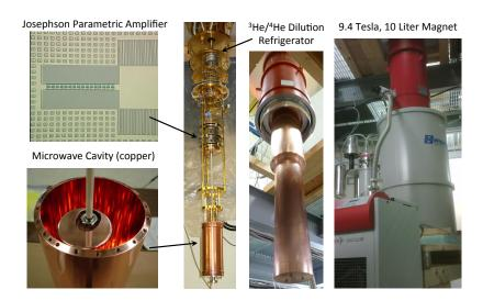
Figure 2: Top left is a microphotograph of the JPA. Bottom left is a photo of the coppercoated, stainless steel resonant microwave cavity with tuning rod inside. To the right of these is a photo of the integrated experiment with the JPA in its magnetic shielding and the cavity on the bottom of the gantry. Next on the right is the same integrated setup covered by thermal shields. Finally, rightmost photo is of the magnet.
