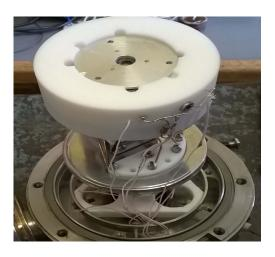
Figure 1: The photo of the beta-spectrometer with the full-absorption Si(Li) detector.
