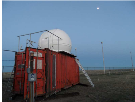
Figure 3: The astronomical dome containing the Lidar, on top of the 20 ft shipping container used in Lamar, Colorado
