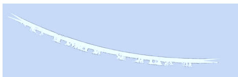
Figure 6: Incorrectly set laser data lead to curvature of the straight tunnel
