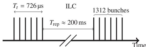
Figure 1: Time structure of the pulses at ILC.
