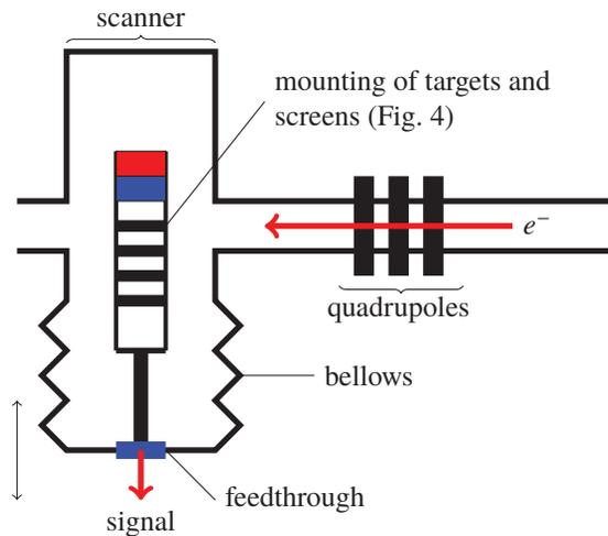
Figure 5: Arrangement to irradiate multiple targets at SF 35.
