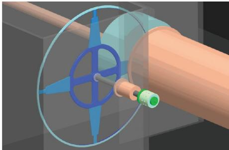
Figure 3: Layout of the positron target. The target is a rotating disc with a diameter of 1 m in order to reduce local stress. Picture taken from [4].
