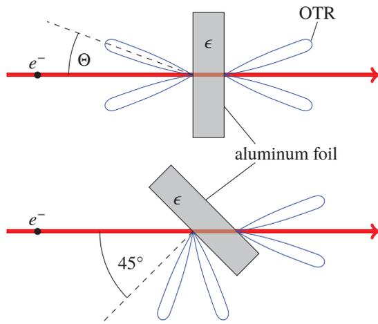
Figure 6: Scheme of emitted OTR (blue) at the aluminum foil perpendicular to the beam and at an angle of 45°. In the latter case, OTR can be observed easily at an angle of  $\approx 90^\circ$ . [6]
